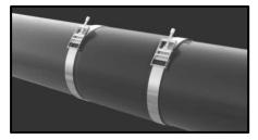
6. Place metal clamps with tensioners on the shrunken ends of the sleeve and use them to tighten the clamps around the shrunken ends of the sleeve. Before proceeding with further activities, wait until it cools down completely (at least 30-40°C).
