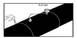
11. The air pressure leakage test according to EN 489.
