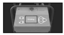
8. Start the welding programme of the electrowelding unit and perform the fusion.
