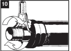
Shrink the end-cap over the step-down and onto the service pipe, keeping the flame moving around the pipe. Stop the heating when the end-cap has fully recovered and its surface has become totally smooth.
