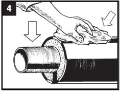
Remove all loose particles from abrading on the jacket pipe and the service pipe by a dry and clean rag. .
