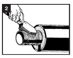
Remove all loose particles from the jacket pipe and service pipe by the steel brush. A deep scars on the jacket pipe shall be removed or scraped flat.
