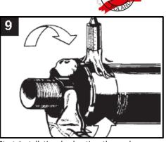
Start installation by heating the end-cap over the jacket pipe first. Move the flame in a circular motion around until the end-cap has fully recovered onto the jacket pipe. Let it cool down a little before shrinking the end-cap over the step-down and service pipe.
