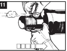
If necessary squeeze the end-cap evenly on the service pipe to relieve the air bulbs. The small wrinkles shall pull themselves out and make the end-cap surface flat again immediately.
