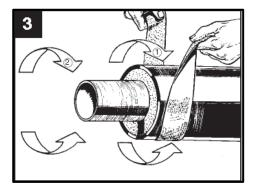
At first abrade the jacket pipe using an abrasive tape, than abrade the service pipe to remove a contamination.
