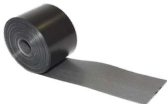
Highest quality closure patches for heat shrink tapes (WPSM-PE, RJS-E). Guarantees secure tightening of tape ends during shrinking. Made of radiation cross-linked high density polyethylene, additionally reinforced with glass fiber. Available in rolls to be cut by user or in ready cut strips.
