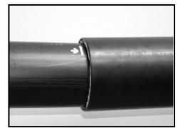
4. Remove the protecting foil from the sleeve and move the sleeve along the jacket pipe to a position between the marks made earlier at step 1.
