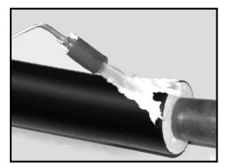
3. The jacket pipe shall be with ca 60°C, if not it shall be heated up by the gas burner.
