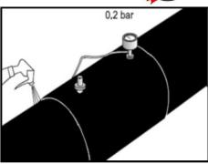
9. The air pressure leakage test according to EN 489.
