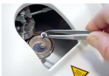
Testing of the thermal stability index (OIT) at CEGA's lab.
