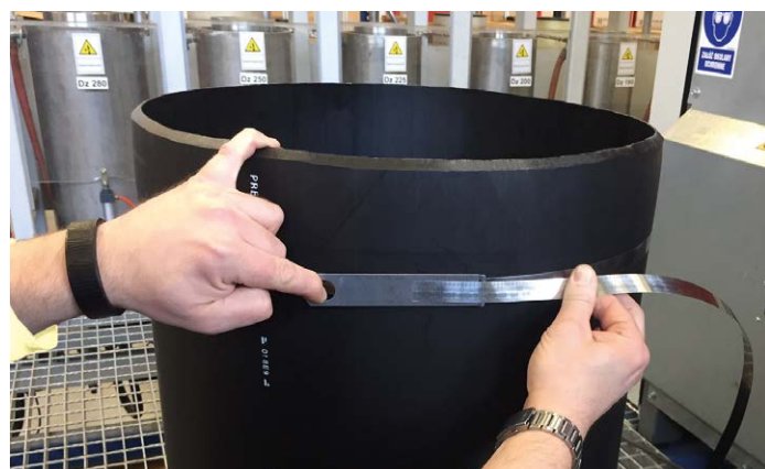
The measurement of the joint's diameter shortly after its thermal expanding.
