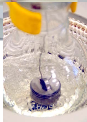
Testing of product's degree of cross-linking in the digestorium (gel content test).
