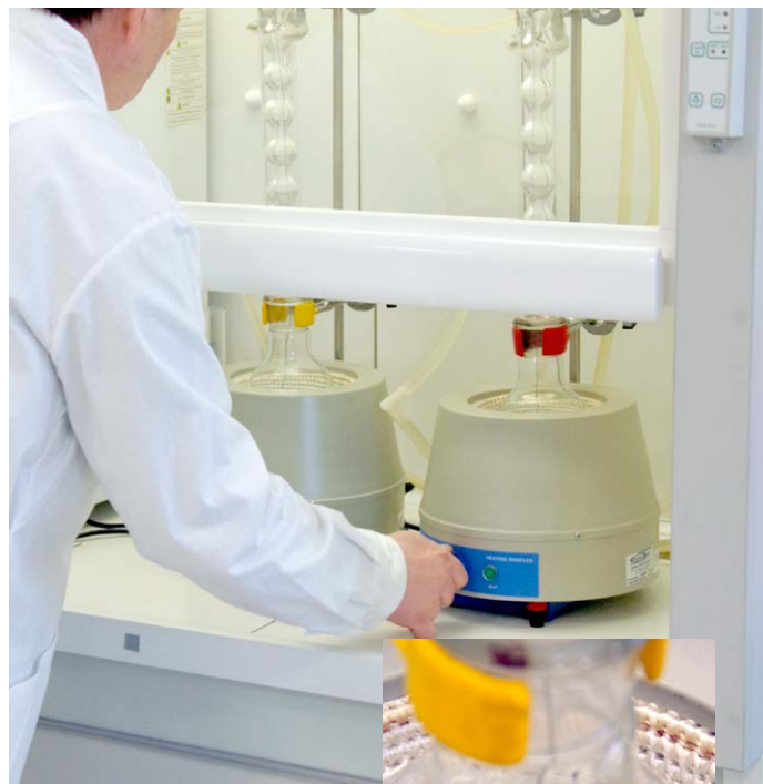
Testing of product's degree of cross-linking in the digestorium (gel content test).
