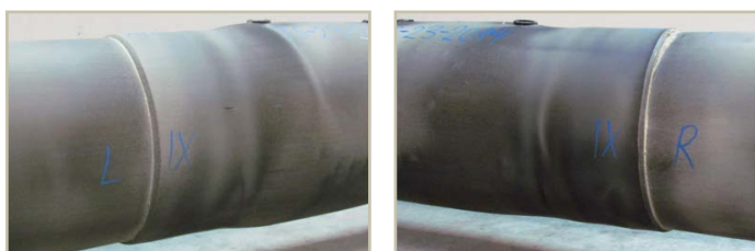
The pictures show the lack of any deformation of MTX2 joints after 1000 cycles in a sand box test (soil stress test) in the accredited HTC Veolia laboratory in Warsaw.
