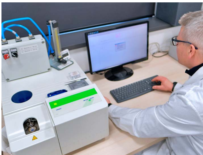
Testing of the thermal stability index (OIT) at CEGA's lab.
